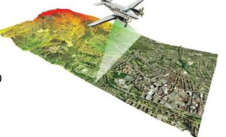
Echoes classified as ground were used to interpolate a digital terrain model (DTM)
